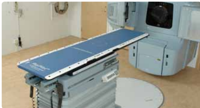
Figure 1. The RayPilot® system together with a linear accelerator.
